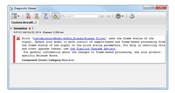
To resolve this error message, reopen Simulink Upgrade Advisor, select the Check model for custom library blocks that rely on frame status of the signal check and click **Run This Check**.
