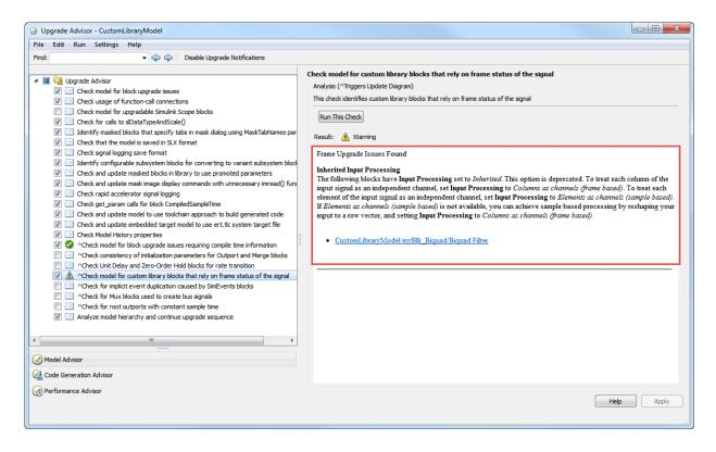
For the CustomLibraryModel/myBlk\_Biquad/Biquad Filter block, the Upgrade Advisor recommends changing Input Processing to either Elements as channels (sample based) or Columns as channels (frame based). To make the change, you update the parameter in the library block, myBlk\_Biquad/Biquad Filter, not in the specific instance of the block in the model. The model now runs successfully.
